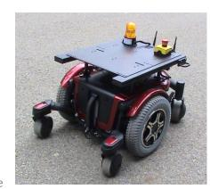
Ethernet interface. Manual control is provided by standard joystick interface. Switching between the two is as easy as flipping a switch.
